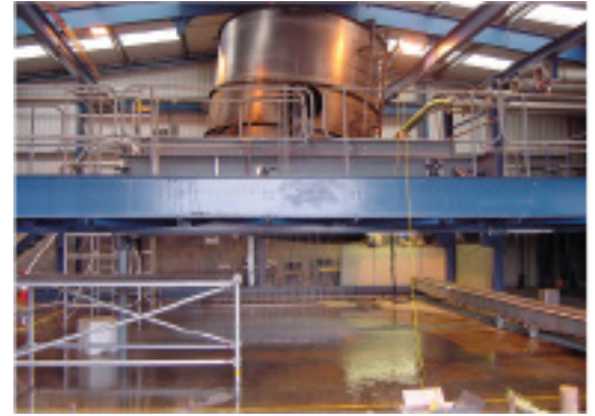
Testing of Model 961 enclosed channel distributor in the Koch-Glitsch test facility simulating wave motion.
