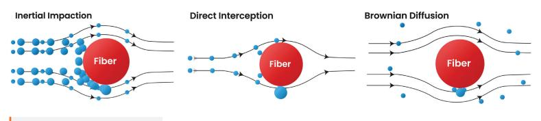
Mechanisms for mist collection on fibers.
