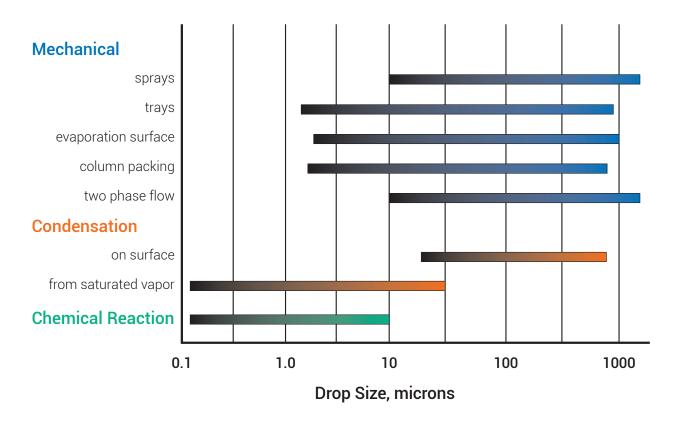
**Mechanical**: Experience shows that droplets generated by mechanical means are commonly 5-10µ and larger in diameter. But a boiling or bubbling liquid surface will form droplets down to just a few microns in diameter.
