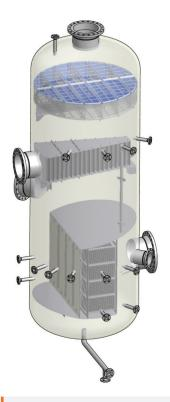
Isometric view of three-phase vertical coalescer/settler.
