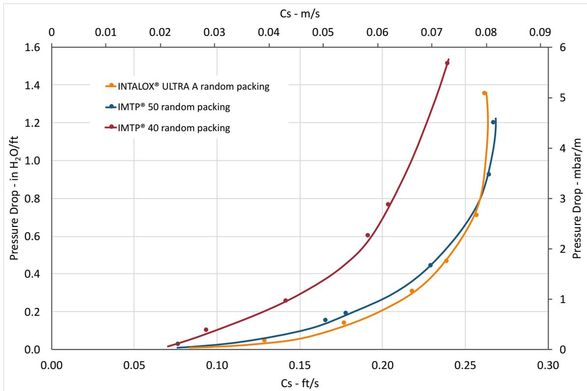
The data above shows that INTALOX® ULTRA A random packing provides efficiency similar to that of IMTP® 40 random packing and capacity/pressure drop similar to IMTP® 50 random packing.
