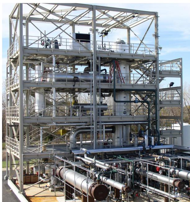
**Figure 2.** Koch Glitsch's 5.5 ft (1.67 m) pilot plant for distillation testing with hydrocarbon mixtures.
